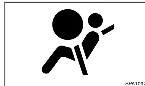
The supplemental air bag warning light, displaying
