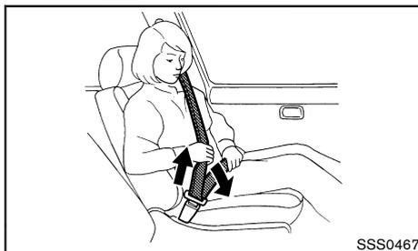
3. Position the lap belt portion low and snug on the hips as shown.
